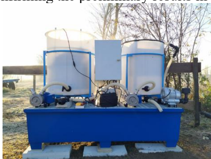
Figure 1: VisioNing pilot plant: from manual to automatic & remote-controlled version
